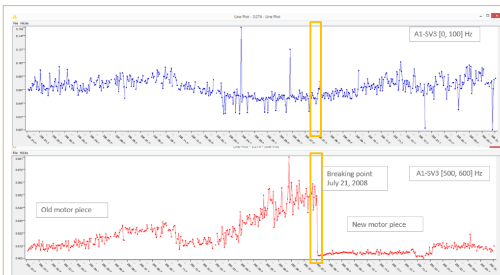
Figure 3. Evolution over time of time series A1-SV31[0, 100] and A1-SV31[500, 600]. The rotor breakdown episode on July 21 st 2008 is easily visible in the higher frequency bands [500, 600] Hz rather than in the lower frequency band [0, 100] Hz. There are 313 such time series in the data set referring to different frequency bands of the original 28 time series.
