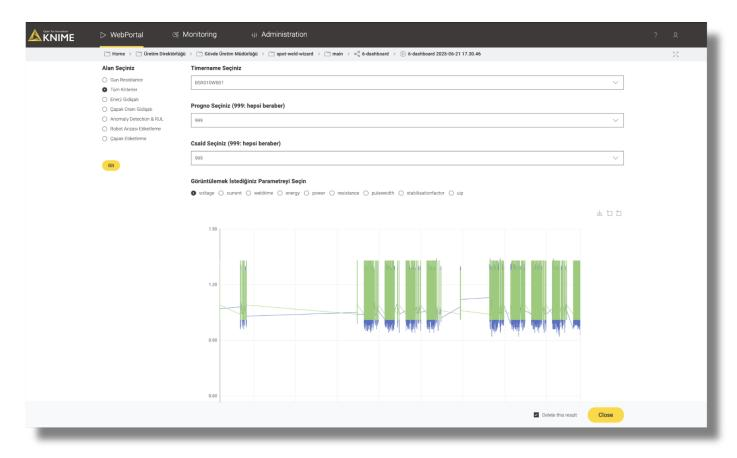
KNIME Data App used by TOFAŞ for real-time monitoring of welding parameters, enabling cross-functional teams to analyze anomalies and validate predictions through an interactive web interface.
